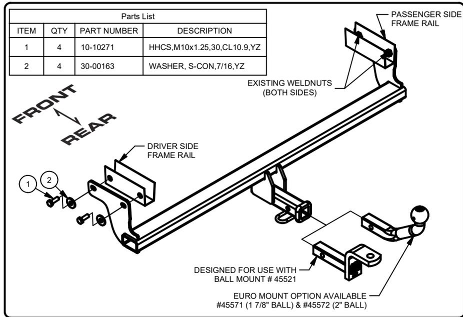
2. Locate and remove the wheel well push pins on each side of the vehicle. Lift hitch into position and secure to the vehicle using (4) M10 hex bolts and (4) 7/16" conical tooth washers. With the hitch in position, reconnect the electrical harness.
