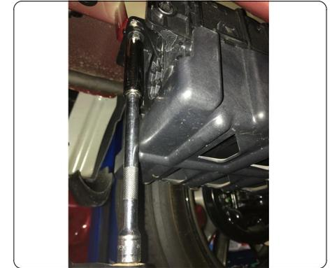
2. On passenger side lower exhaust by removing (2) exhaust isolators, using isolator removal diagram, to expose heat shield. Remove (4) speed nuts to lower heatshield from frame rail.
