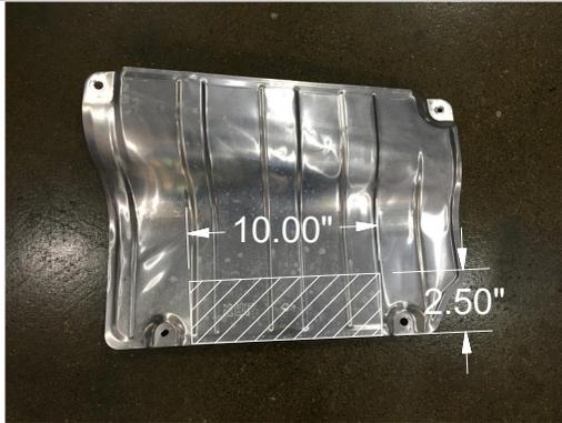
4. Enlarge forward most attachment hole on both sides using a die grinder. Use hole enlargement diagram as a reference.
