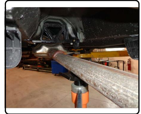
2) On some model years the wheel well plastic on each side of the vehicle near the frame rails will need to be trimmed to provide a flush fit for the hitch side plates. Be sure to avoid the vehicle brake lines when cutting the plastic away.
