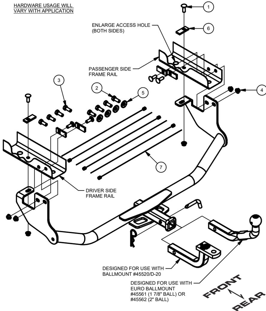
1) Lower rear exhaust hangers from one location on each side of the vehicle. For ease of installation, the exhaust can also be lowered in one location at the front center of the vehicle. This location will need to be lowered slowly and supported from underneath during install. Caulking may need to be trimmed around side mounting holes if present.
