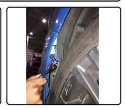
2. Remove bumper beam by removing (6) nuts using 13mm socket, (3) on each side. Set bumper beam aside for reinstallation.
