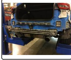
5. Mark out 2.25" x 2.00" section using masking tape. Trim rear fascia and trim heat shield as shown in the trim diagram using aviation shears.
