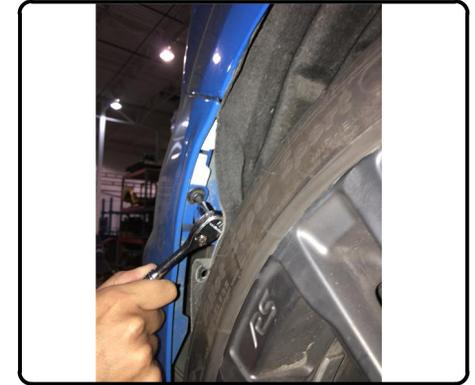
2. Remove bumper beam by removing (6) nuts using 13mm socket, (3) on each side. Set bumper beam aside for reinstallation.
