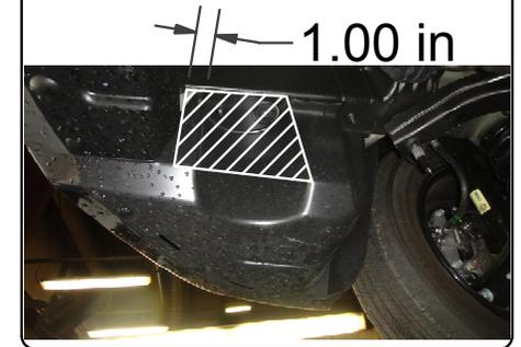
2. Raise hitch into position by placing the passenger side into position first. Secure hitch by loosely installing (4) M10 bolts and conical toothed washers as shown. Torque hardware to 48 ft-lbs and reinstall underbody panel.
