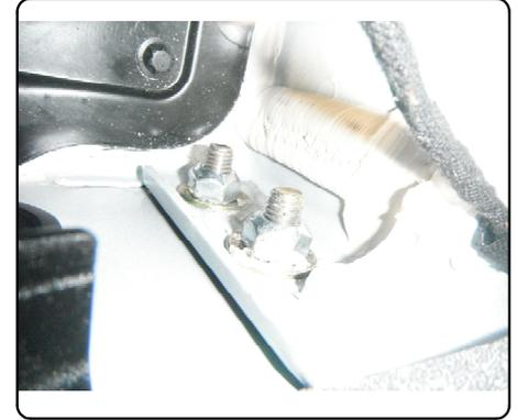
22. Torque (4) inner M10 nylock nuts to 45.2 ft-lbs. Torque outer (4) factory nuts on bumper beam studs to 31.6 ft-lbs.
