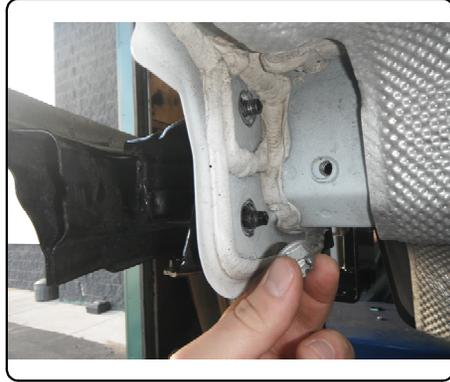
20. Insert (4) supplied M10 hex bolts with (4) M10 washers through bumper beam, hitch and vehicle.
