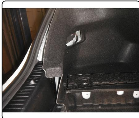
9. Remove (3) hex nuts which secure the taillight using an 8mm socket. Remove (1) hex nut using a 10mm socket. Repeat removal of (4) nuts on other side.
