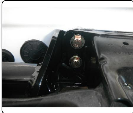
21. Apply silicon around base of (4) bolts on inside of vehicle. Insert (4) M10 washers onto bolts and secure with (4) M10 nylock nuts using 17mm sockets.
