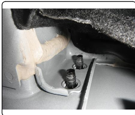
17. Cut off the heads of (4) inner bumper beam studs and knock studs off using a hammer. Clean holes so supplied M10 bolts can be inserted and paint any bare metal.
