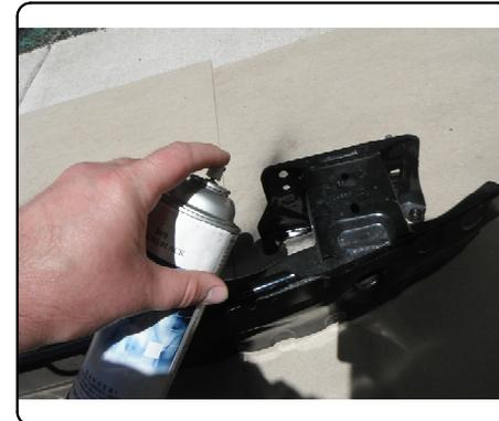
18. Apply silicon on outside of vehicle around (4) inner mounting holes. NOTE: This is important to prevent exhaust fumes from entering the vehicle.
