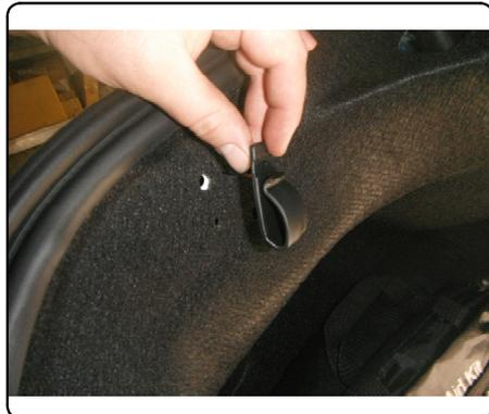
5. Remove (1) tie down per side using a T40 torx tool.
