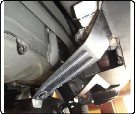
2. Raise hitch into position and install supplied fasteners as shown. Torque all 3/8" fasteners to 37 lb-ft and all 5/8" fasteners to 180 lb feet. Re-install remaining bumper fascia tabs to original positions.
