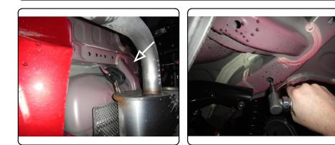
2. Fishwire the 1/2" bolts and spacers into the frame rail as shown above.
