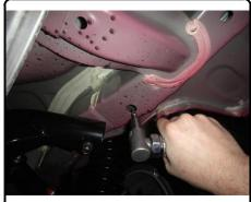
2. Fishwire the 1/2" bolts and spacers into the frame rail as shown above.
