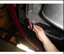
4. Torque all 5/8" fasteners to 210 lb-ft. Torque all 1/2" fasteners to 110 lb-ft.
