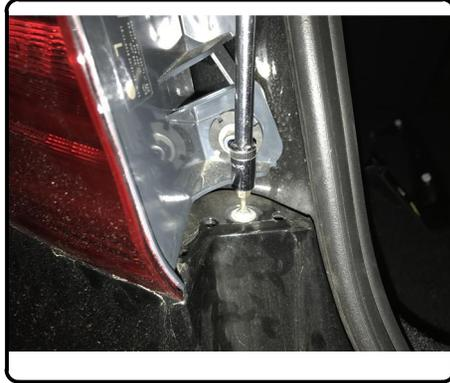
4. Remove (2) bolts using 10mm socket from each tail light. Carefully remove rear bumper fascia. **NOTE:** To ease fascia removal, begin from outside and work towards the center of the vehicle.
