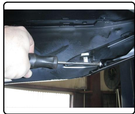
2. Using a 12mm socket, remove the (8) bolts attaching the bumper assembly to the rear face of the cabin. Lightly pull the lower fascia away to remove the bumper beam and return flange bolts to vehicle owner.
