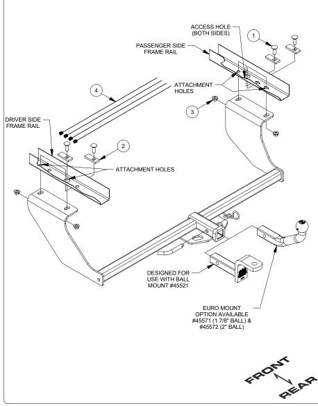
1. Fishwire (2) 7/16 carriage bolts and (2) CM-SP2 spacers through the access holes and into the attachment holes in each frame rail.
