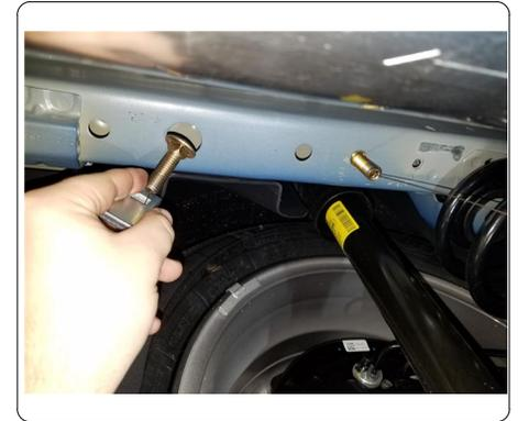
2. Raise hitch into position feeding fishwires through holes in hitch. Remove fishwires and secure hitch with (4) 7/16 hex flange nuts.
