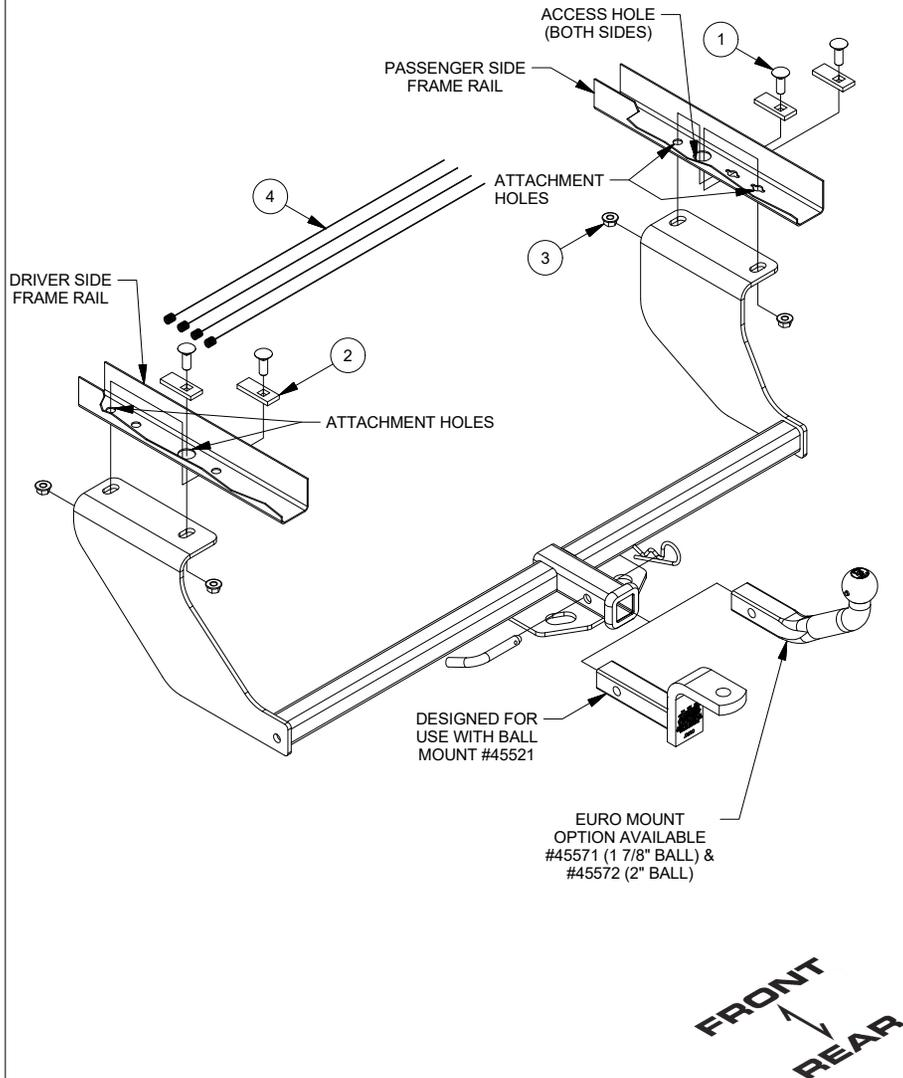
1. Fishwire (2) 7/16 carriage bolts and (2) CM-SP2 spacers through the access holes and into the attachment holes in each frame rail.
