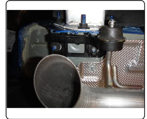
2. Temporarily remove the heat shield using a needle nose pliers to remove the (6) retention nuts. Trim heat shield following contours as shown removing a 3" x 3" square using Trim Diagram below as reference.
