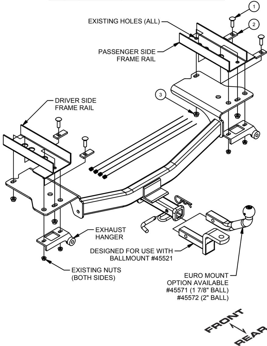
1. Lower exhaust by using a 13mm socket to remove (2) nuts from each exhaust hanger. There is a plastic clip on the exhaust hanger that needs to be pushed out of the way to allow the exhaust to be lowered.
