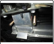
6. Raise hitch into position, guiding bolts through slots in hitch. Loosely secure hitch into position using (4) 1/2" hex flange nuts.
