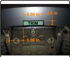
5. Insert (2) 1/2-13 x 4.5" in each bolt plate. Gently pull fascia down and place bolt plate with bolts on top of each bumper beam extension.
