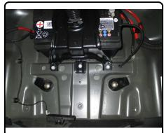
8. Torque (4) hex flange nuts securing 1/2-13 x 4 1/2" bolts to side plates to 75 ft-lbs. Torque (2) hex flange nuts securing mounting plate to 110 ft-lbs.
