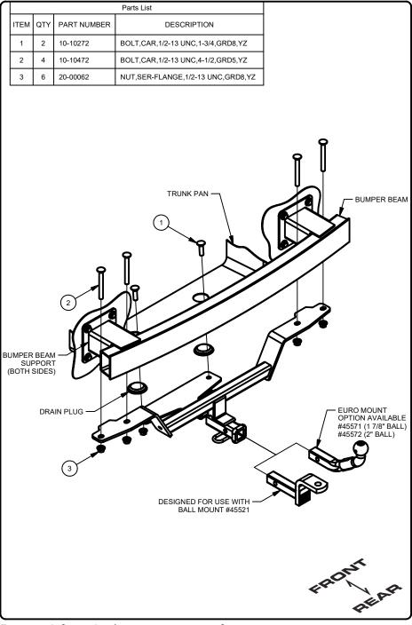
1. Using a 10mm socket remove (2) hex nuts holding rear plastic fascia to bottom of trunk pan. Save (2) nuts for reinstallation in STEP 9.
