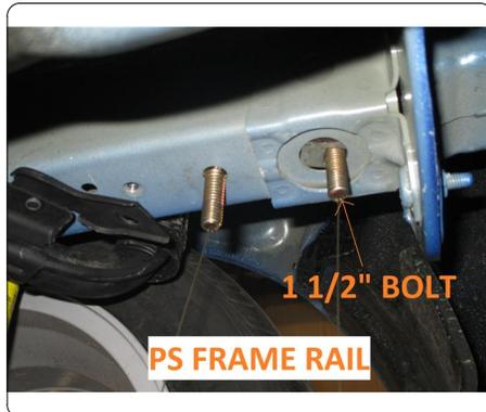
7. Pull fascia down and raise hitch into position by sliding passenger side plate under plastic tab as shown below.
