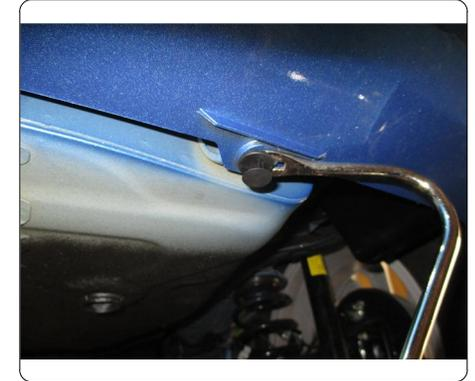
2. Remove one (1) M8 bolt on passenger side frame rail using a 13mm socket. Pull plastic away from frame rail as shown in photo below.
