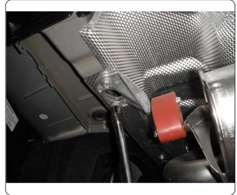
2. Raise hitch into position and temporarily secure to existing weldnuts in the frame rails using (4) M8-1.25 hex bolts and (4) 3/8" conical toothed washers. Using the hitch as a template mark drill location on both sides. Lower hitch and drill holes.
