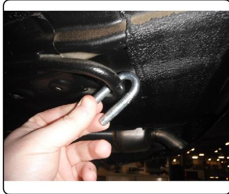
4. Raise hitch into position and slide u-bolt through holes in hitch.
