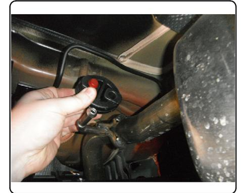
2. Temporarily remove driver side underbody panel by removing (3) clips using a flat head screwdriver and (4) nuts using a 10mm socket.
