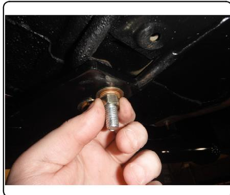
5. Torque M10 hardware to 48 lb-ft (if applicable), M8 hardware to 23 lb-ft (if applicable) and 3/8" hardware to 26 lb-ft.
