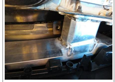
6. Raise hitch into position, aligning the slots in the hitch with the holes in the nut plates. Loosely secure the hitch into position using (4) 1/2-13 x 5" hex bolts and 1/2" conical toothed washers (2) each side.
