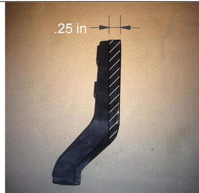
5. Reattach trimmed fascia brackets. Gently flex the rear fascia and place nut plates on top of the bumper beam supports.
