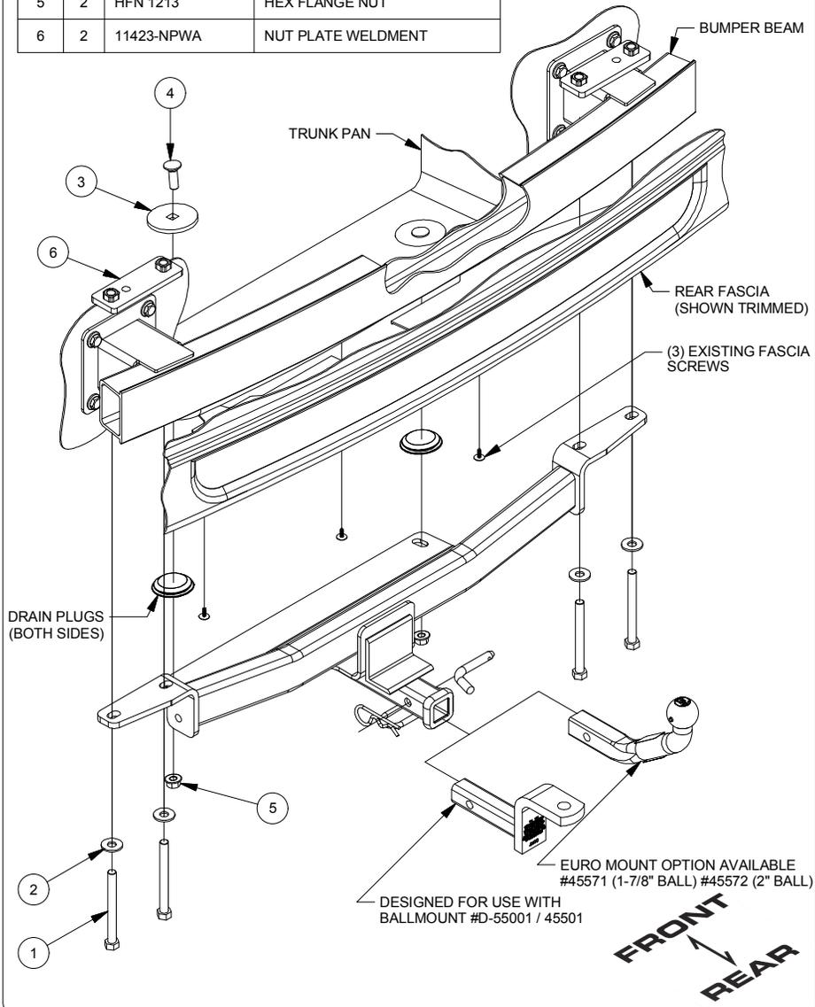
1. Remove the (3) fascia screws holding the rear plastic fascia to the bottom of the trunk pan. Retain (2) screws for reinstallation in Step (9) and return (1) screw to owner. **Note:** For 2016 models remove (2) inboard T-30 screws that retain exhaust tips (1) on each side, and remove exhaust tips.
