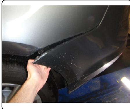
5. Remove (7) M8 bolts from the bumper beam using a 13mm socket. Remove the bumper beam from the vehicle by lifting it up and then away from the vehicle.
