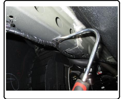
2. Enlarge access hole forward of tow loop on passenger side frame rail to allow 7/16" carriage bolts and CM-SP11 spacers to pass through.
