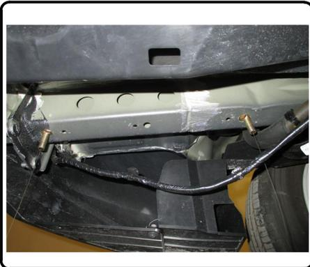
5. Raise hitch over exhaust into position and pull fishwires and carriage bolts through side plates. **Note:** Feed fishwires through mounting holes while raising hitch. Remove fishwires from carriage bolts and secure hitch with 7/16" flange nuts.
