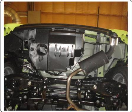
2. Remove the factory tow hook and hardware from vehicle and return to owner.
