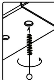
To remove debris from weldnuts in frame, spray lubricant or compressed air into hole. For heavy debris, use a small wire brush. (Be careful not to damage threads).
