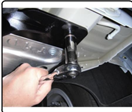
5. Torque all 7/16" carriage bolts to 59 ft-lbs and 7/16" U-bolt to 25 ft-lbs. Raise and secure exhaust back into position.
