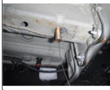
6) Reinstall the exhaust heat shield and raise the hitch with the exhaust back into positon. Loosely install the supplied 1/2" hex flange nuts.
