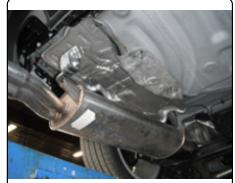
2) Remove the exhaust heat shield from the driver side and the plastic underbody panel on the passenger side. Keep fasteners for later re-installation.
