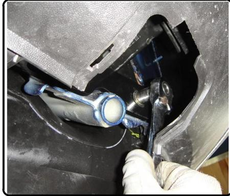
4. Place (2) 1/2" carriage bolts into the square holes in the chain loop plate. Reattach exhaust and secure bumper cover using the (2) outer fasteners removed in Step 1. Note: Center attachment is no longer accessible.
