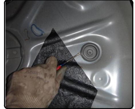
6. Use silicone caulk (or equivalent) to seal the tire well plug hole from exhaust fumes and water by putting a bead around each hole inside the spare tire well. Place a 11410-SP spacer onto each hole and put a bead of caulk around each square hole. Install a 1/2" carriage bolt into each hole.
