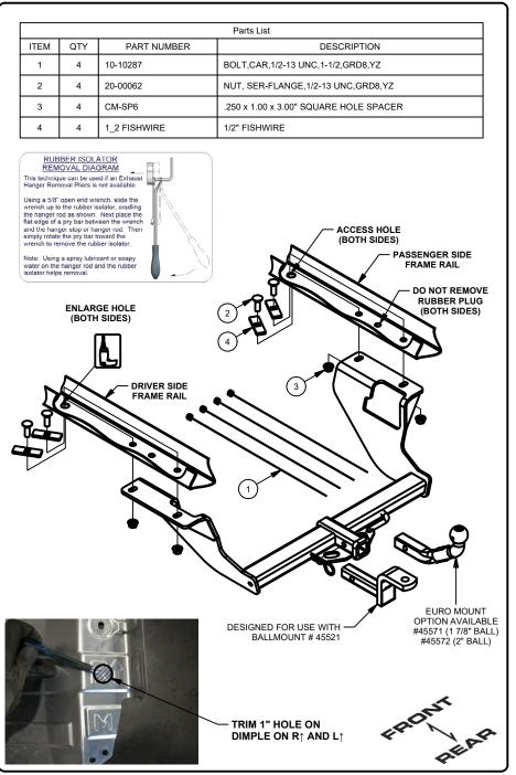
1) Lower exhaust by removing (5) rear rubber isolators.
