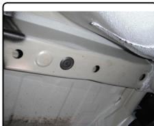
4) Fishwire the 1/2" hardware through the access hole into position on both sides, as shown below. Reinstall heat shield with (3) of the fasteners, leaving out the one between the mounting holes.
