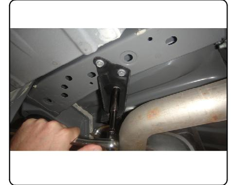
2. Enlarge the access holes to allow the carriage bolts and spacers to pass through.
