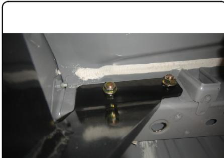
5. Torque all 7/16" hardware to 70 ft-lbs. Re-attach muffler brackets removed in Step 1. Torque all M8 muffler bracket hardware to 23 ft-lbs.
