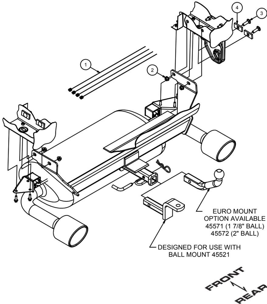
1. Lower exhaust by removing (6) bolts from the muffler brackets, retain bolts for reinstallation.
