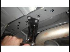
2. Enlarge the access holes to allow the carriage bolts and spacers to pass through.
