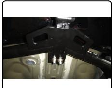
4. Place the SP22 spacer on top of the driver side plate and secure hitch to the frame rails using 7/16" flange nuts.
