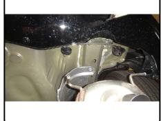
2. On the driver side, reverse fishwire a 7/16-14 x 1 1/2" carriage bolt and SP2 spacer through the existing hole. On the passenger side, reverse fishwire a 7/16-14 x 1" carriage bolt and SP2 spacer through the existing hole.
