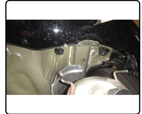
2. On the driver side, reverse fishwire a 7/16-14 x 1 1/2" carriage bolt and SP2 spacer through the existing hole. On the passenger side, reverse fishwire a 7/16-14 x 1" carriage bolt and SP2 spacer through the existing hole. **Note:** The longer carriage bolt must be installed on the driver side.
