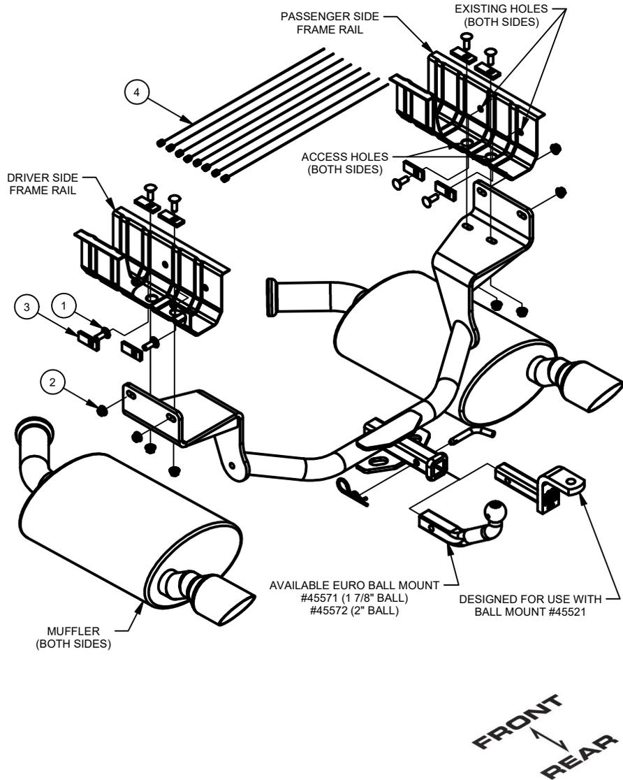
1. Lower exhaust by removing (6) M8 bolts, from hanger brackets, with a 13mm socket.
