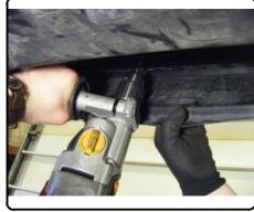
Fishwire 1/2"-13 x 2" carriage bolts and SP6 spacers through the end of the bumper beam and into holes drilled in Step 4. See Fishwire Technique Diagram
