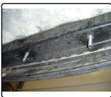
6. Raise hitch back into position and secure with 1/2"-13 flange nuts. Torque all 1/2" fasteners to 110 ft-lbs.
