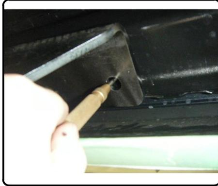
4. Lower hitch and drill hole locations with 9/16" drill bit. **Note:** Drilling a small pilot hole prior to the 9/16" hole will ease this process. Another option is to drill a small pilot hole and enlarge with a die grinder.
