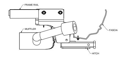
INSTALLED HITCH POSITION
