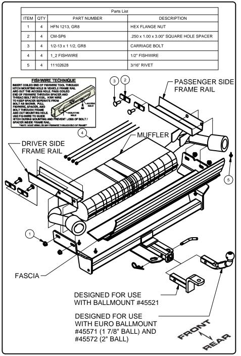
1.) Remove corner plastic shield from each side of the vehicle by using an 8mm socket to remove 3 bolts and a phillips screwdriver to remove 1 nut (each side).
