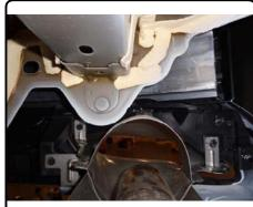
4.) Remove plastic fascia by drilling out rivets with a 3/16" drill bit (each side). Remove 3 bolts from center fascia with a 10mm socket. Unclip fascia around exhaust outlets and gently pull fascia away from the vehicle.
