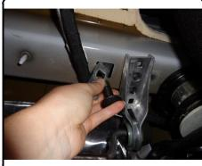
6.) Raise hitch into position and secure with 1/2" flange nuts. Note: Seam foam may need to be trimmed for proper mounting hole alignment.
