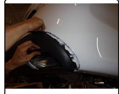
5.) If lowered, raise exhaust and secure back into position.
