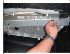
4. Fishwire 1/2" bolts and spacers into position through enlarged hole and out rear holes. Reverse fishwire 1/2" bolts and spacers into enlarged holes. (Both sides)
