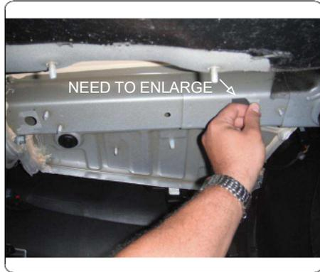
4. Fishwire 1/2" bolts and spacers into position through enlarged hole and out rear holes. Reverse fishwire 1/2" bolts and spacers into enlarged holes. (Both sides)
