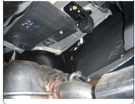
2. Temporarily remove heat shield(s) by removing (3) fasteners with a 10mm socket and remove plastic underbody panel (if present) by removing (4) plastics fasteners and (2) fasteners with a 10mm socket.
