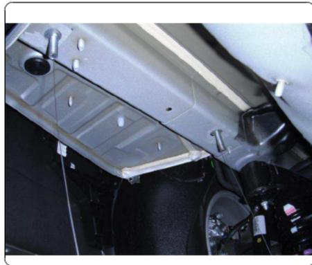
5. Raise hitch into position and attach to frame using 1/2" flange nuts.
