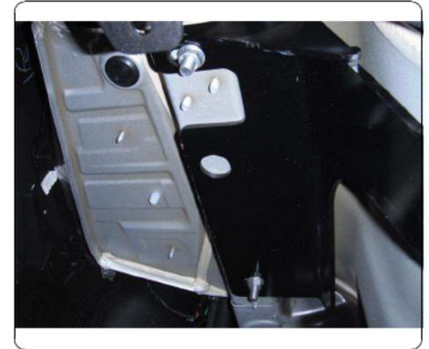
6. Torque all 1/2" hardware to 110 ft-lbs. Reinstall heat shield(s) and leave rear most fastener off. Raise exhaust back into position. If underbody panel was present, trim and reinstall. (See TRIM DIAGRAM)
