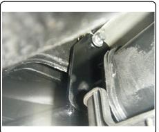
6. Install 1/2" carriage bolt with spacer through tow hook and hitch, lightly tighten with 1/2" flange nut provided.
