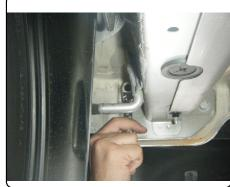
5. Position hitch in place and use the (3) 8mm supplied bolts and conical washers, lightly tighten.
