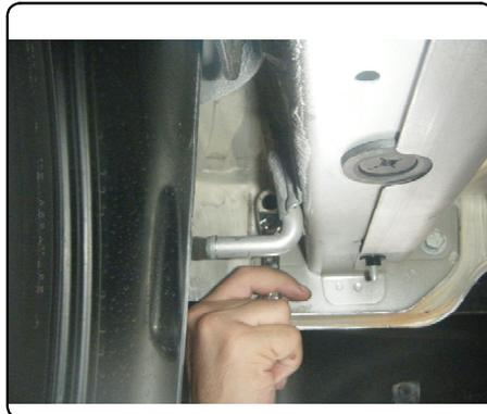
5. Position hitch in place and use the (3) 8mm supplied bolts and conical washers, lightly tighten.
