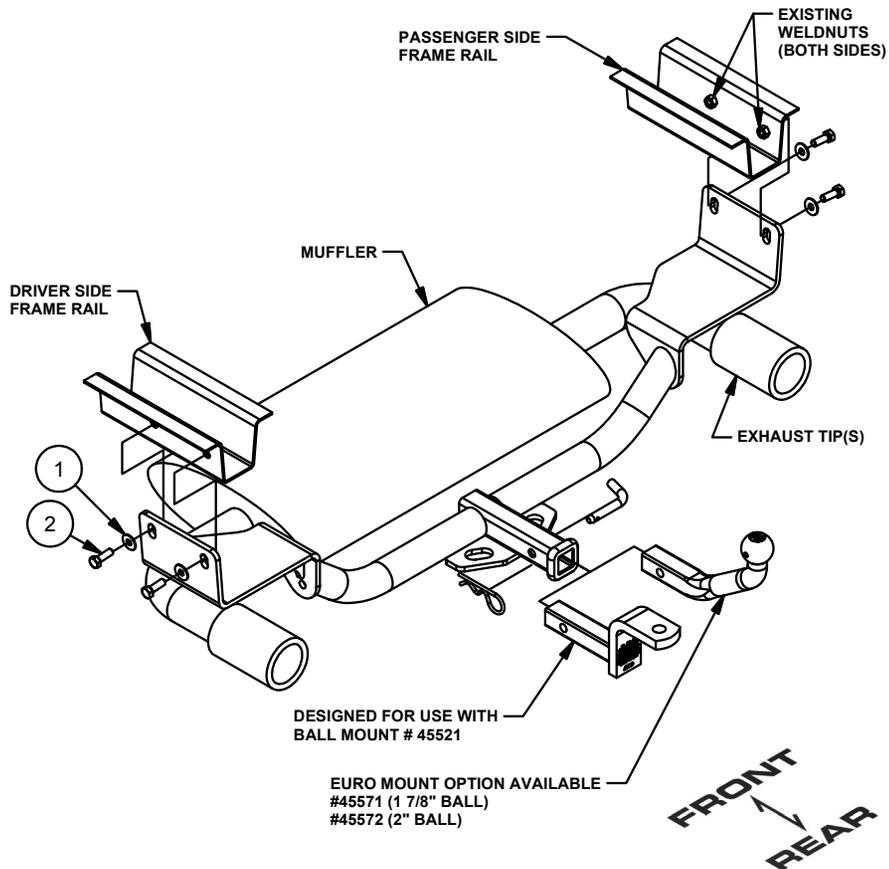
1. Lower exhaust by removing (2) rubber isolators from the exhaust side leaving the isolators attached to the vehicle. Exhaust will be supported by the rear axle. (see Rubber Isolator Removal Diagram)
