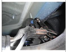
2. Raise hitch into position over exhaust.
