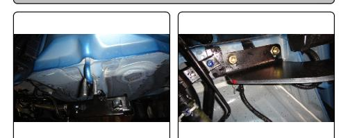
4. Torque all 7/16" hardware to 70 ft-lbs. Torque all 3/8" hardware to 45 ft-lbs.
