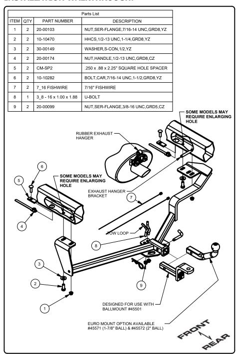
1. Lower rear rubber exhaust hanger from frame attachment. (See Rubber Isolator Removal Diagram)
