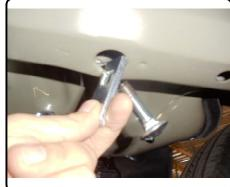
5. Insert 1/2" handle nuts through access holes. (Both sides)
