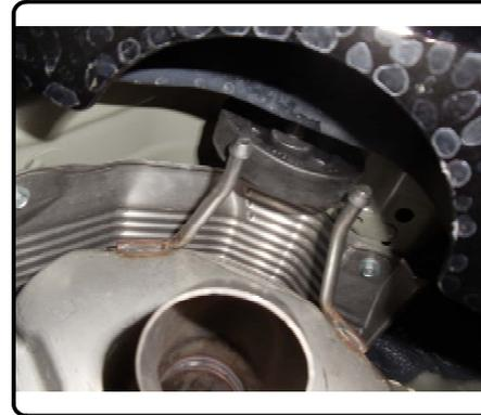
**RUBBER ISOLATOR REMOVAL DIAGRAM**
