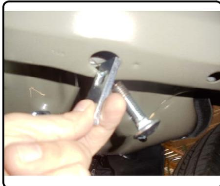
5. Insert 1/2" handle nuts through access holes. (Both sides)
