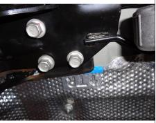
4. Raise the hitch into position against the frame rails and reinstall the exhaust hanger brackets using the (6) M12 bolts. Note: The hitch is sandwiched between the frame rails and the exhaust hanger bolts.
