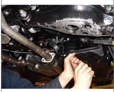
Remove the (6) hex flange bolts securing the exhaust hanger brackets with a 17mm socket and remove the brackets (each side). Save the bolts and brackets for reassembly.
