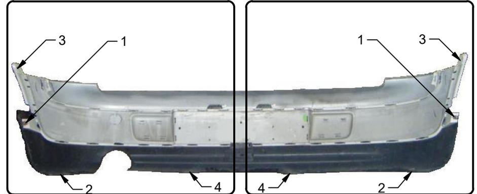
2. Using a phillips screwdriver remove fastener 1 from inside the rear wheel well. **Note:** If needed you may remove the rear wheels to access screws.
