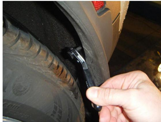
3. Using phillips screwdriver, remove fastener 2 from the bottom of the bumper near the rear wheel well. The second photo shows the optional mud flap removed.
