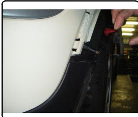
5. The first photo shows the lower fender flare tabs released. Using an offset phillips screw driver or wrench with a phillips driver bit remove hidden fastener 3 behind the fender flare.
