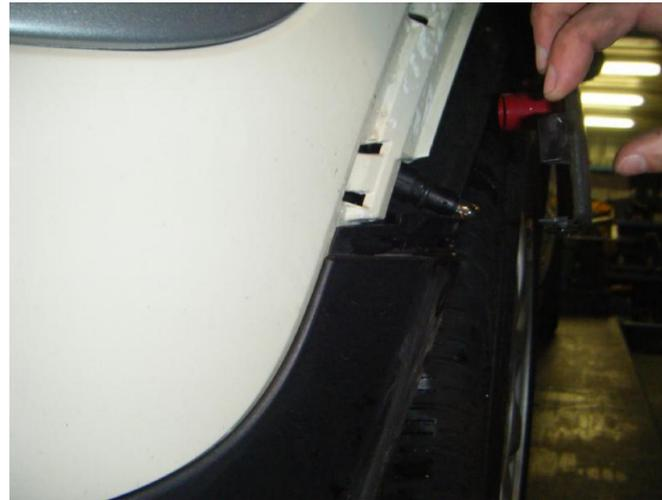
5. The first photo shows the lower fender flare tabs released. Using an offset phillips screwdriver or wrench with a phillips drive bit remove hidden fastener 3 behind the fender flare.
