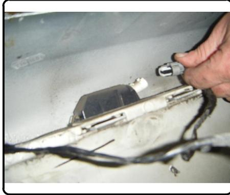
8. The first photo shows the bumper cover removed, exposing the aluminum bumper beam. Using a flat blade screwdriver remove the (7) wiring harness clips from the bumper beam.
