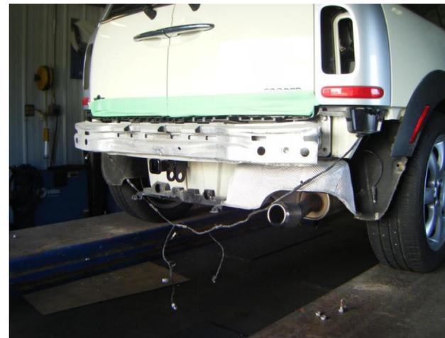
12. An access hole will need to be drilled through your bumper cover to allow access to the receiver tube. Mark your drill location by measuring down from the bumper cover lip 3-3/4" and center by using the dimple in the license plate cover. Using a 2-1/2" hole saw drill through the license plate holder and bumper cover. When drilling make sure not to drill through the sensor bracket or loose wiring.
