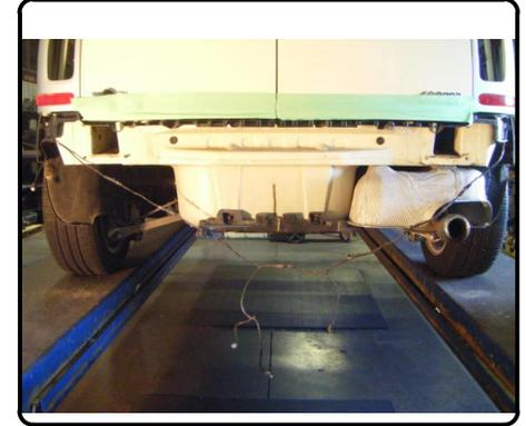
10. Raise hitch into position by aligning the holes and weld studs on the car with the holes in hitch. Sandwich the hitch between the bumper beam and the rear of the car.
