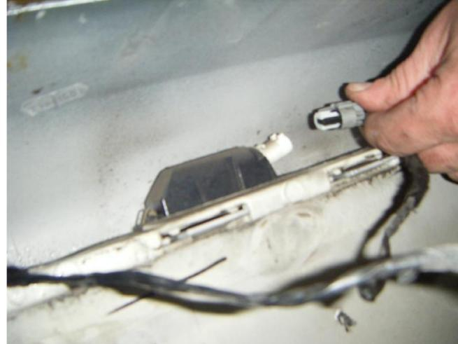
8. The first photo shows the bumper cover removed, exposing the aluminum bumper beam. Using a flat blade screwdriver remove the (7) wiring harness clips from the bumper beam.
