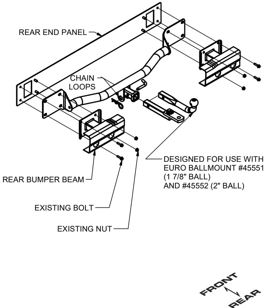
1. Remove (8) fasteners that secure the bumper cover.
