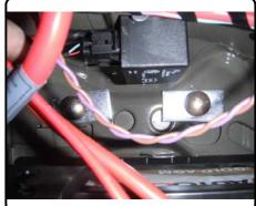
6) Torque all 1/2" fasteners to 110 lb. - ft. Trim underbody panel as required and reinstall onto vehicle. Slide battery back into position and reinstall carpet and trunk contents removed in step 3
