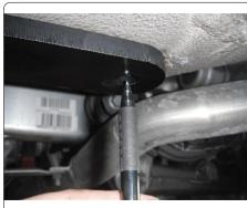
4) Remove tail bracket and drill both holes from below the vehicle using a 17/32" drill bit (for 1/2" fasteners). Reinstall the tail bracket to the hitch using (2) 1/2" - 13 X 1 1/4" carriage bolts and 1/2" hex flange nuts.
