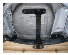
5) Apply silicone caulk to the SP4 spacers and remaining 1/2" carriage bolts and install into the trunk pan and tail bracket as shown and loosely install the remaining 1/2" hex flange nuts.
