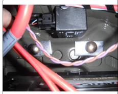
6) Torque all 1/2" fasteners to 110 lb. - ft. Trim underbody panel as required and reinstall onto vehicle. Slide battery back into position and reinstall carpet and trunk contents removed in step 3
