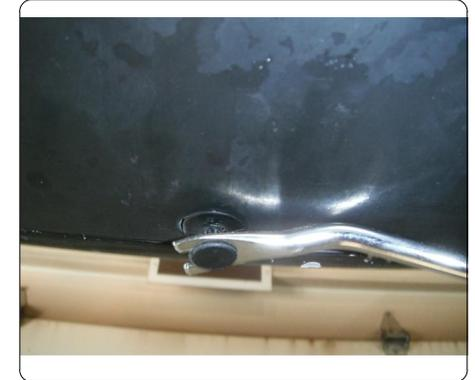
2) Fishwire (2) 1/2" -13 X 1 1/4" carriage bolts and (2) SP6 spacers into the existing holes in the bumper beam as shown in the diagram above. Raise hitch into position and loosely install the 1/2" hex flange nuts.
