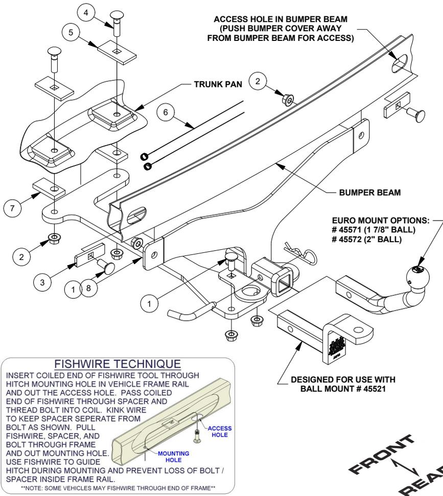
1) Remove underbody panel that attaches the bumper cover to the trunk pan using a 10mm socket and plastic rivet remover. Save for later reinstallation.
